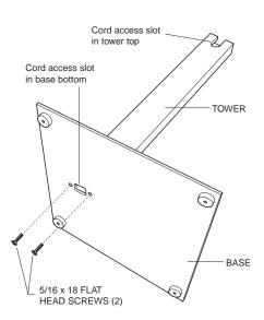
(STEP 1) Screw Tower to Base with (2) 5/16 x 18 Round Head Screws. Note that it is important which direction the slot in the Tower Top faces depending on the application desired. See Steps 2A and 2B for possible applications.
