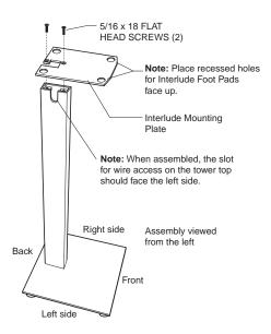
STEP 2B Interlude IL10 – When used with Interlude IL10 speakers, the assembly process is the same, regardless of LEFT or RIGHT placement.
