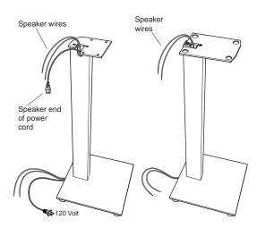
STEP 4 Insert speaker end of power cord in cord access hole in base and feed it up and out through the top. Run the speaker wires in the same manner.
