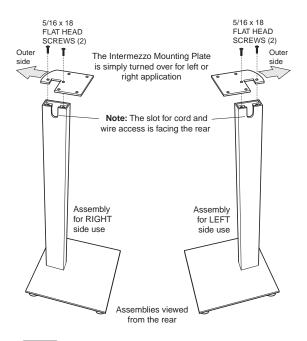
STEP 2A Intermezzo 2.6 – When used with Intermezzo 2.6 speakers, the rounded edge of the Mounting Plate should face the outer side of the stand assembly; the same side as the decorative side panel on the front of each Intermezzo speaker.
