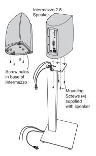
STEP 5A Intermezzo 2.6 – Place the Intermezzo speaker on its mounting plate and secure with (4) screws (provided with the speaker).
