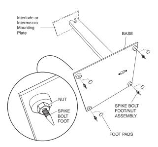
STEP 3 The floor stand includes both spikes and felt pads. For installations on a carpet, we recommend the use of the spikes as this will provide maximum stability and acoustic isolation. For applications where there is a floor surface that may be damaged by the spikes, felt pads are also provided. The Spike Feet are comprised of a Spike Bolt and a Nut that tightens to lock the Spike Bolt in place.
